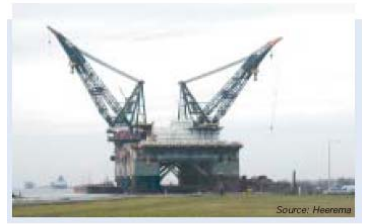
Thialf, Crane Ship 6 x 5.5 MW Thruster Drives (ACS 6000)
